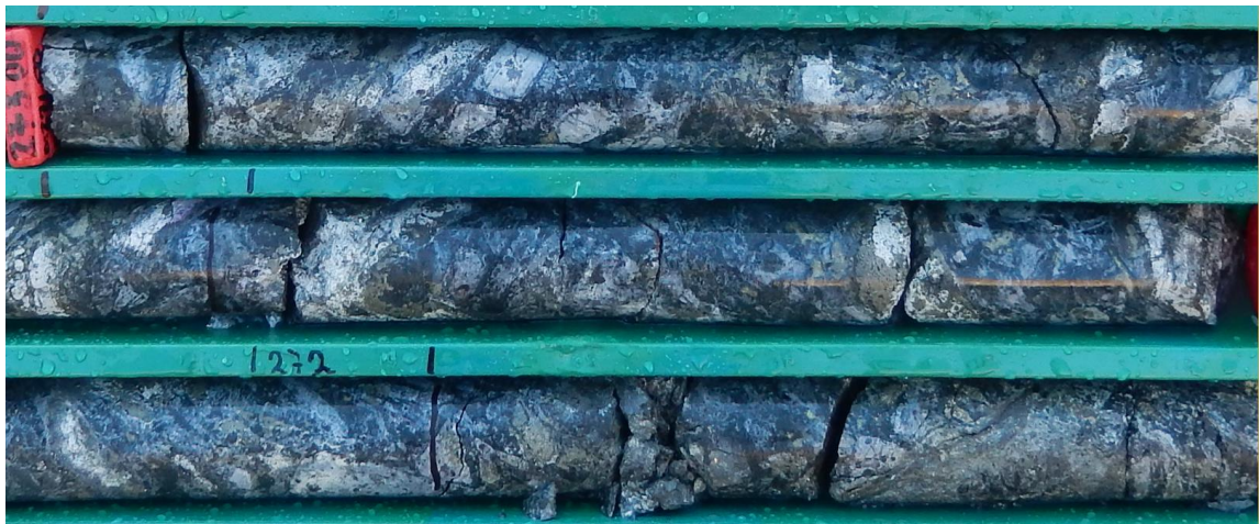
Figure 1: Partial core tray photo showing core between 271m and 273m: Complexly altered and veined sulphide-bearing tourmaline breccia similar to the Clint Breccia intersected in CH-DDH012.
