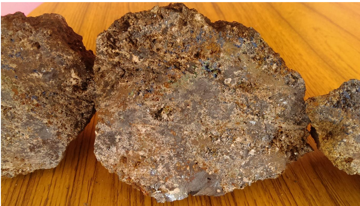
Figure 1: Rock grab sample Y308RK showing blue and green secondary copper minerals in a matrix of quartz magnetite and goethite.
