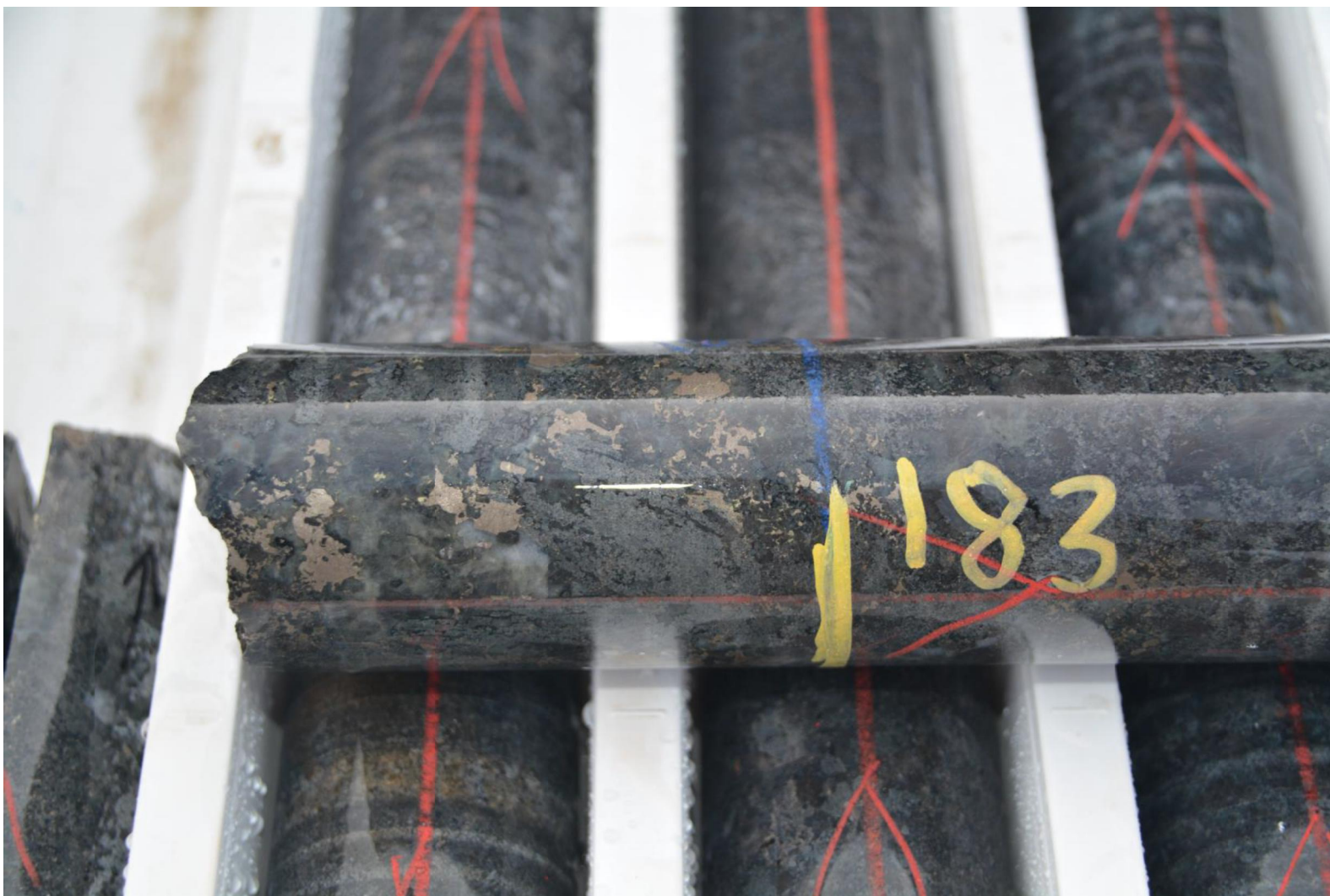
PLATE 1.0 – NQ Core from MRDD002 at 183.00 metres downhole. Blebby sulphides in coarse grained olivine norite. Sulphides include pyrrhotite, pentlandite, chalcopyrite and pyrite. Hole located approximately 130m along strike from newly identified conductor T19C01 at Target 19.
