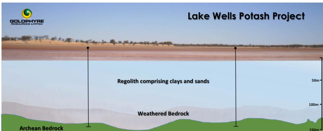
Figure 3: Lake Wells Potash Project, Schematic cross section with proposed drill hole trace demonstrating blade refusal penetration through regolith and deep palaeochannel section
