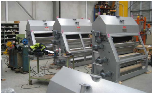
Figure 4: Magnetic Separators during fabrication, now installed at Picton
