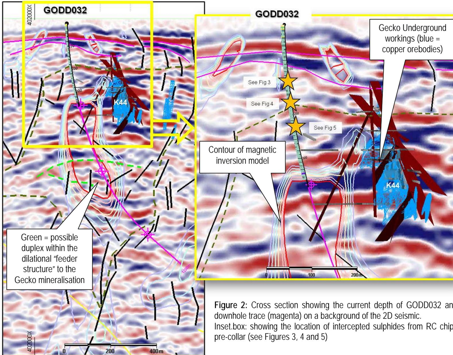
**Figure 2:** Cross section showing the current depth of GODD032 and downhole trace (magenta) on a background of the 2D seismic. Inset box: showing the location of intercepted sulphides from RC chips pre-collar (see Figures 3, 4 and 5)
