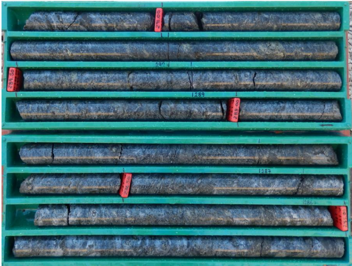
Figure 1: Complete core tray photo of CH-DDH013 from 284m to 291.4m. The tourmaline-sulphide rich nature of this breccia is similar to the Clint Breccia, which contains copper, gold, silver and molybdenum (see ASX announcement 27 May 2014, ASX announcement 23 July 2015).
