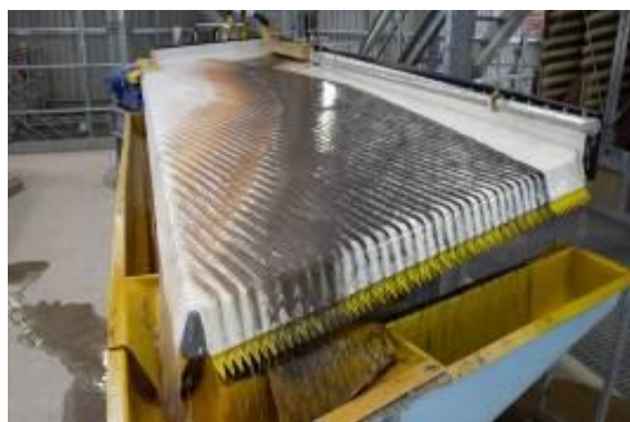
Image 8: Shaking table with black tungsten concentrate
