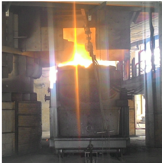
A03 Main Workshop furnace 6 tapping in progress
