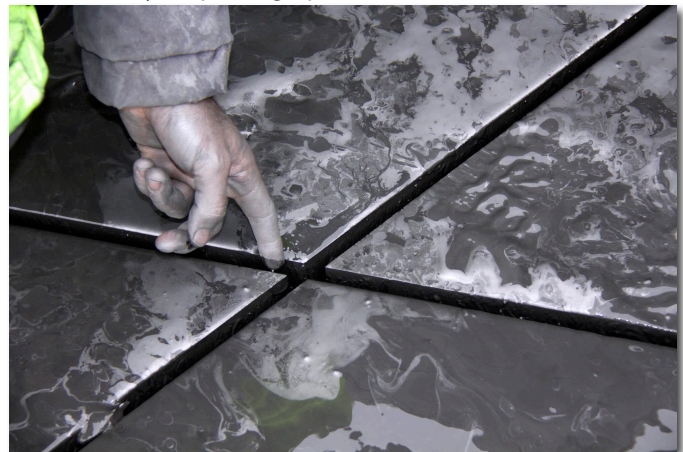
Figure 4. The amenability of the mining technique to precisely and efficiently shape the graphite ore blocks is evident.
