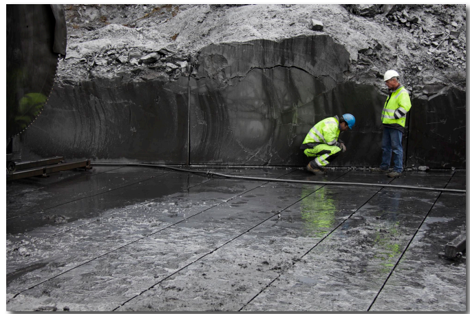
Figure 3. Talga's Project Manager Kane Freeman and Group Geologist Simon Coxhell inspecting the trial mine ore bench.
