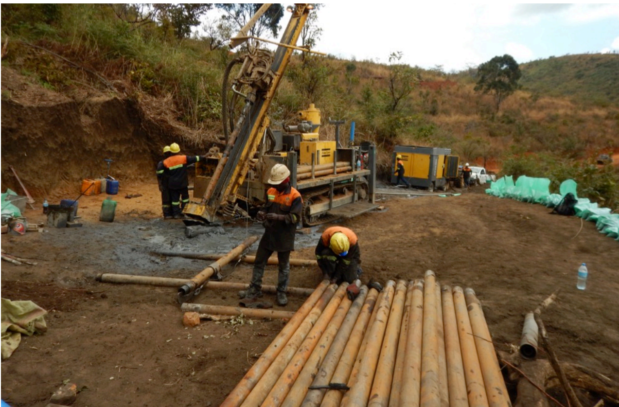
Photo 4, above. Portion of the 230m trench extension to Cascade trench C1, showing near surface graphitic schist outcrop. Photo 5, below. RC drill rig at Epanko north
