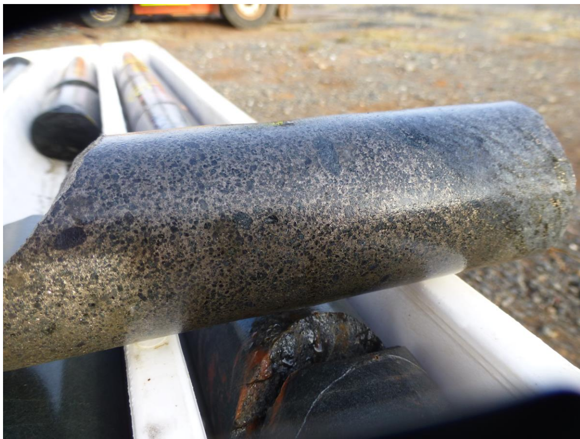
Figure 3: Semi massive to net textured pyrrhotite in mafic granulite / gabbro
