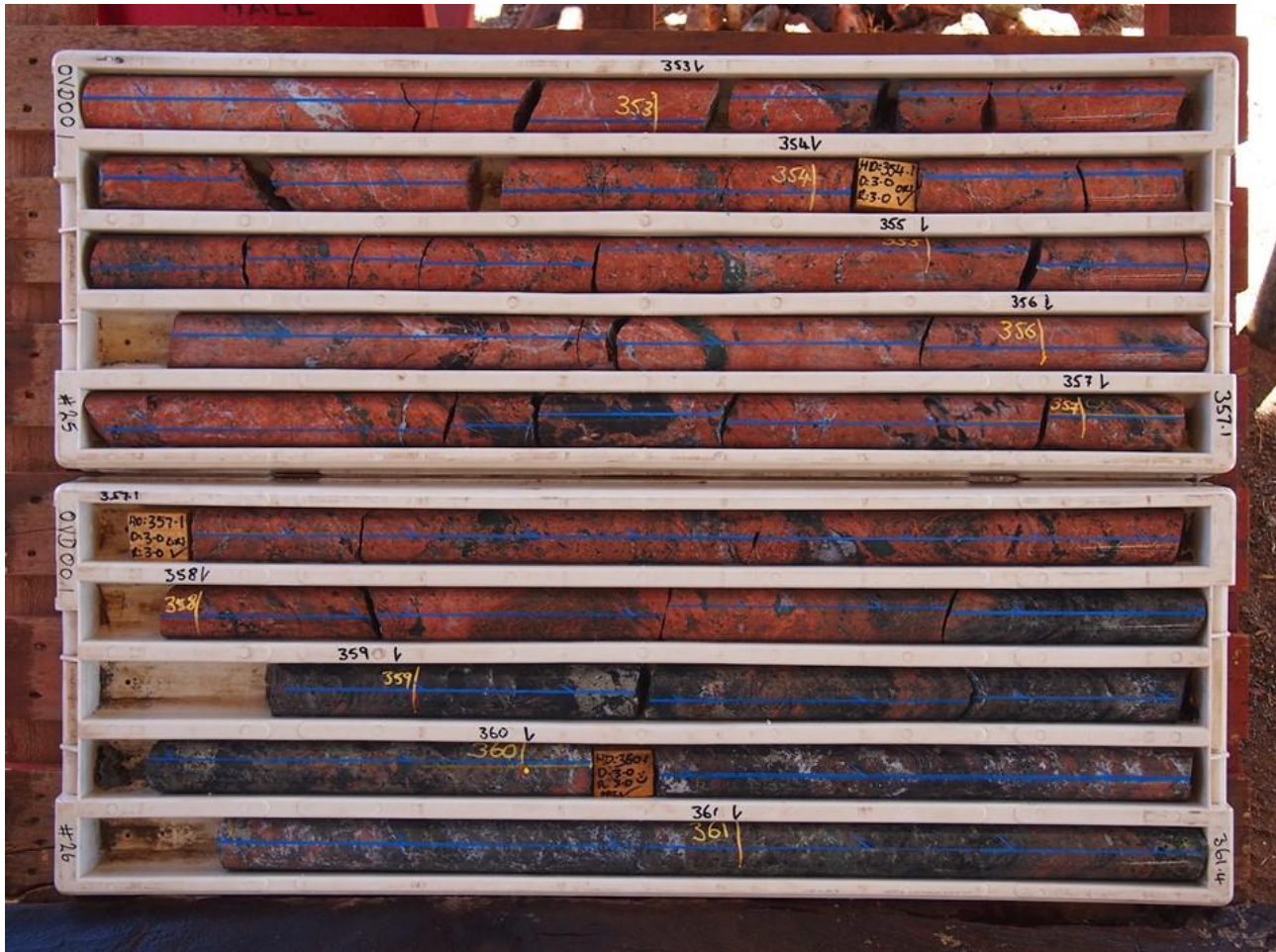
OVD001 – Footwall Alteration
