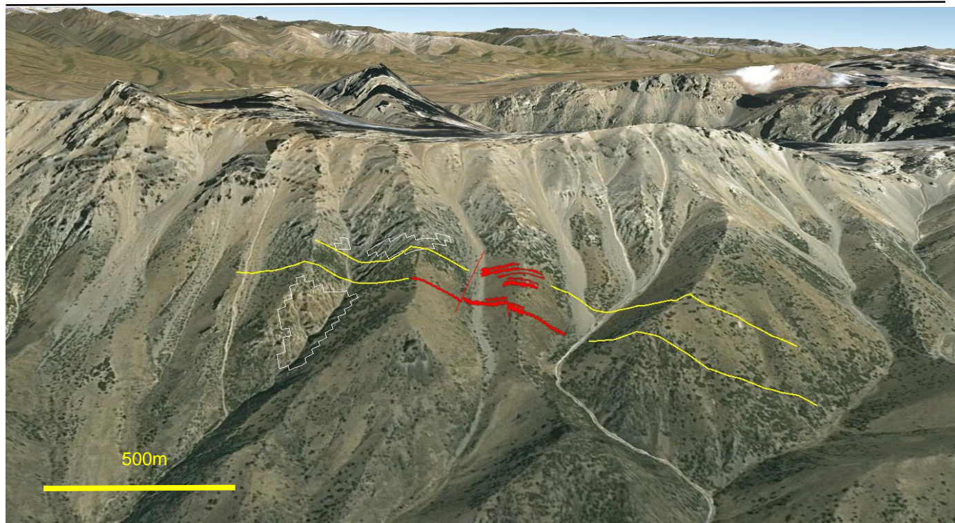
Figure 3 The surface outcropping Aucu high grade gold resource (red outlines) with exploration in 2015 planned to test the extensions shown in yellow.
