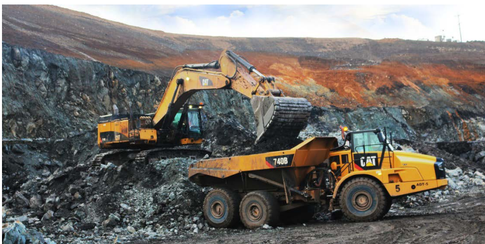
Figure 1: Mining activities in the Siana open pit, Western wall cut-back
