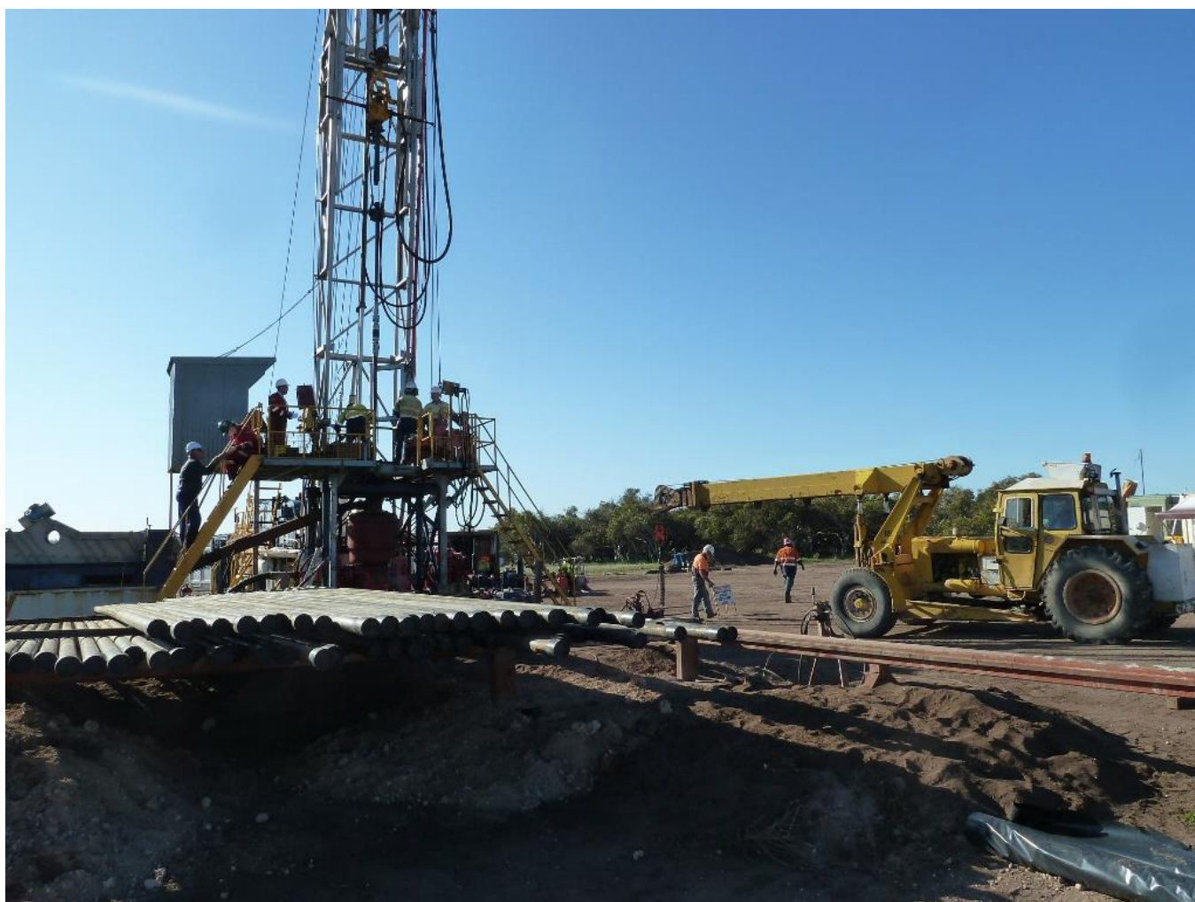
DCA Rig #6 at the Dunnart-2 wellsite with 3 ½” tubing for the completion racked on the pipe racks prior to running in hole and commencing testing operations
