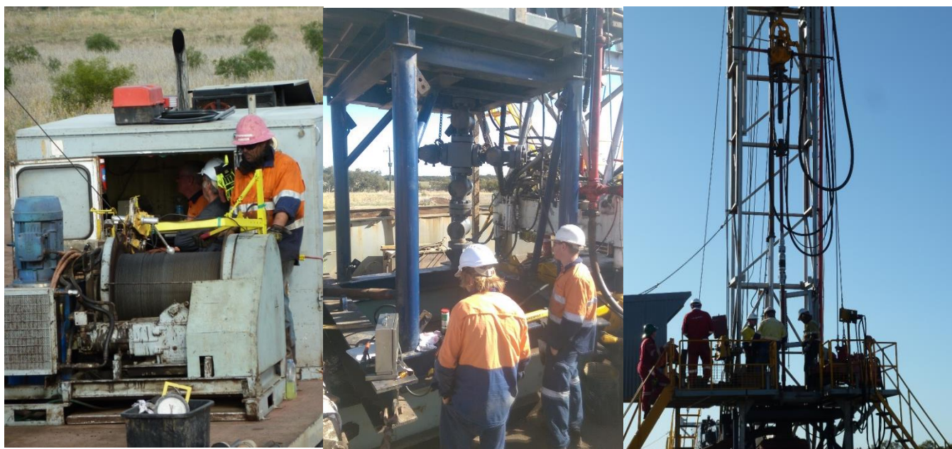
Westlog wireline services (left) with DCA roughneck assisting, TKM preparing to secure the production Christmas tree (middle) and completion engineers and DCA hands overseeing the running of completion equipment prior to testing through the tree (right)
