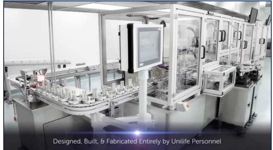
Assembly line for the Unifill Finesse™ at Unilife's facility in York, PA
