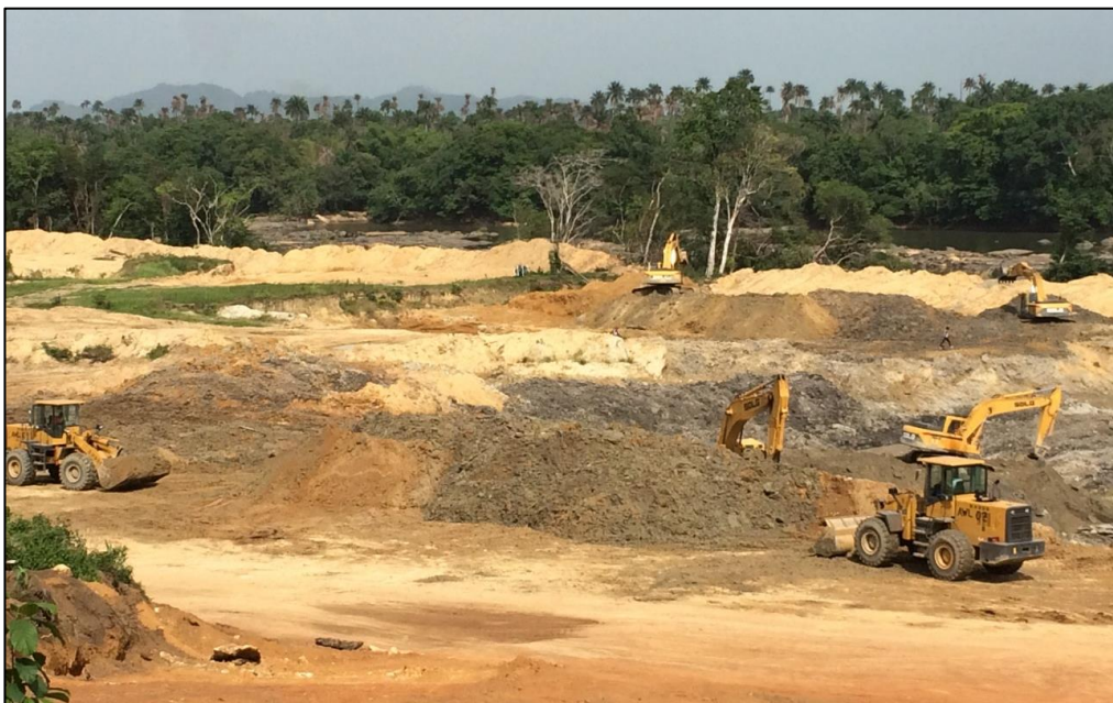
Figure 6. Pre-stripping and mining activities in the Golu trial-mining pit, Baoma District. Note: a previous bulk-sample trench, excavated to test for mineralisation, lies at the top of the photo (green, grassy area trending left to right.) The tree-line marks the bank of the Sewa River.
