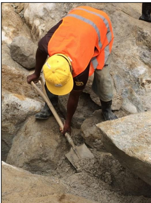
Figure 8. Supervised manual bedrock sweeping between gullies and crevices. Due to the high specific gravity of diamond, these bedrock perturbations contain much of the basal gravel mineralisation.
