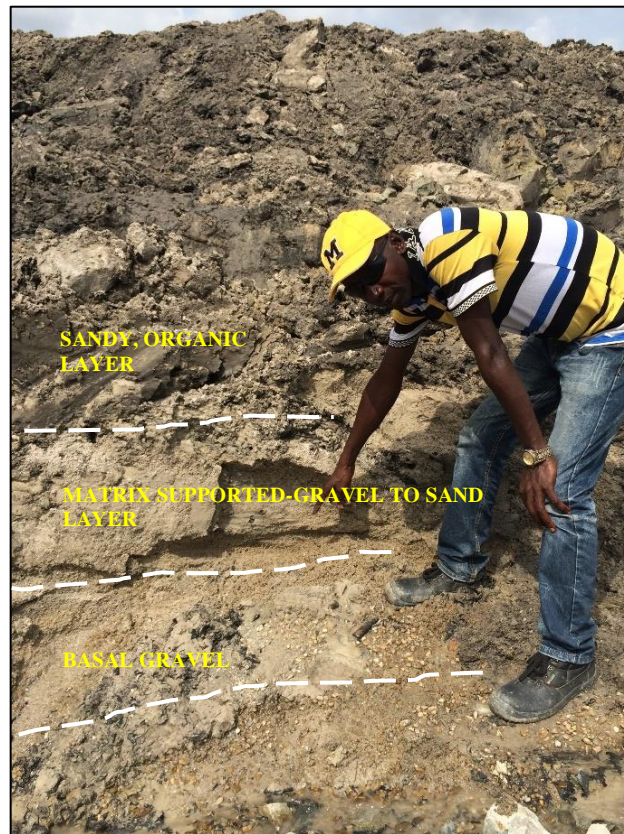
Figure 7. The Lower Terrace ore horizon, Golu trial-mining pit. The basal gravels (note white quartz vein clast assemblage) are enriched in grade, relative to the buff coloured, overlying sandier unit (the '5' - note bedding planes). The dark-grey excavated material (at top) is a localised sandy organic unit overlying the '5' and deposited as a slack-water layer as the river gradually abandoned its course.
