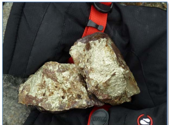
Figure 4: Examples of massive chalcopryite copper ore from Pahtohavare. Samples, likely from the Southern Deposit, were located on the mines' waste dump during a recent field trip.
