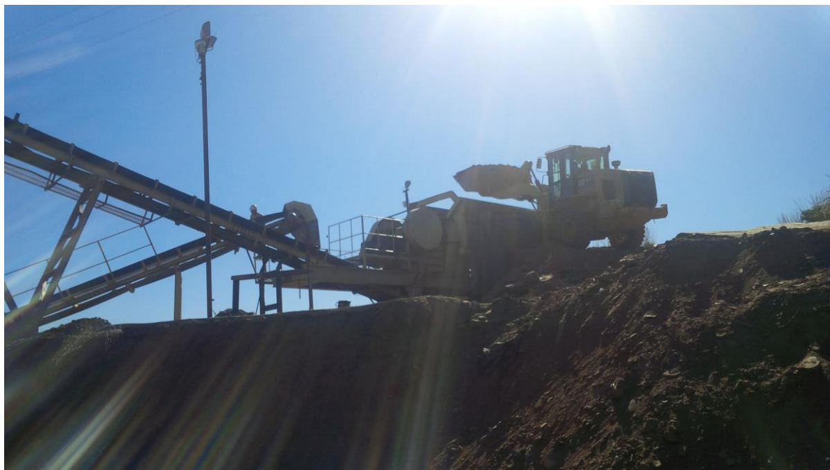
Ore being fed into the primary crusher at Premier
