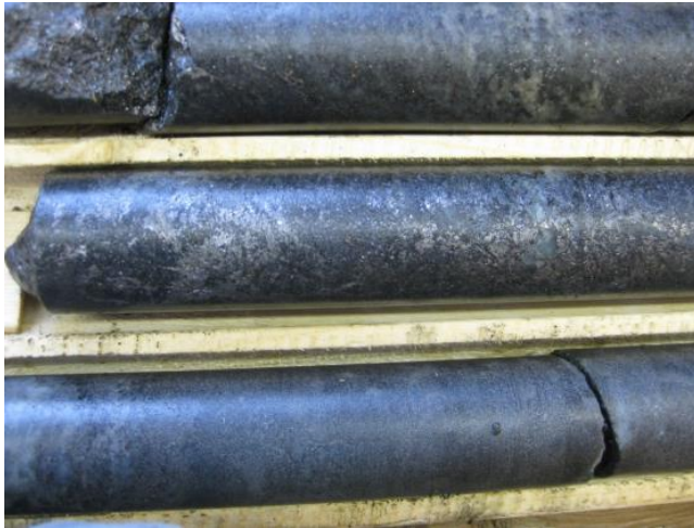
Figure 2: Jumbo and large flake graphite present in drill core from maiden drilling program
