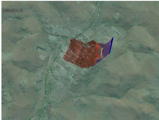
Plan view of Belvedere with drilling and mineralisation. Belvedere Fault mineralisation in blue, this is open to the north. Other lodes constrained to the Dolerite host and are only open down dip
