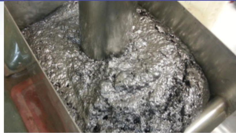
High Grade Concentrate - Final cleaner concentrate from an initial rougher cleaner test
