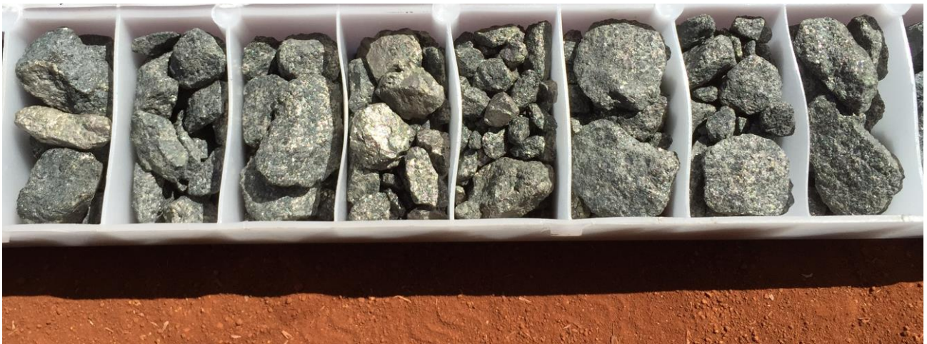
Figure 1. RC chips from the massive and matrix sulphide zone, from 50-58m in hole DMRC003
