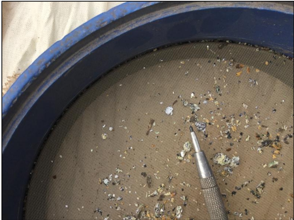
Figure 5. Assessment on friable weather material hand crushed between fingers – note a mix of gangue minerals present however several pieces of jumbo flake are present – black nib on scribe is 3.5mm
