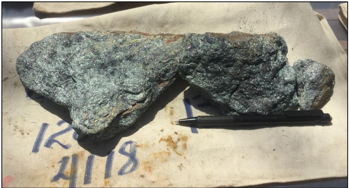
Figure 7. 13_C Sample 1.2m from surface, high grade graphite sericite schist 10 -15% VGE
