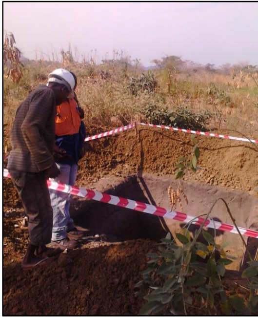
Figure 3. Typical trench dug over primary VTEM anomaly – notice the graphitic soil and bedrock
