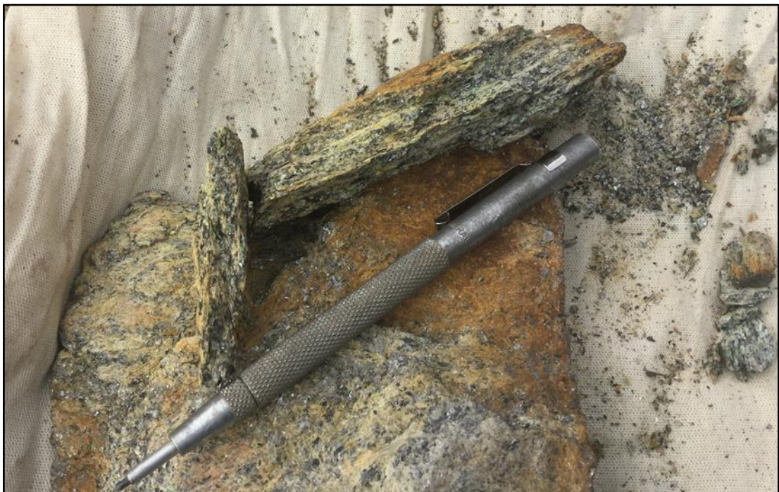
Figure 4. Graphitic Schist outcrop: grade estimate 10% graphite with weak sericite alteration
