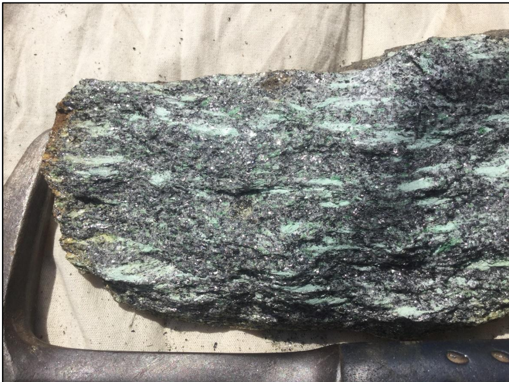
Figure 6. High grade rock chip sample – Graphite – Sericite - Quartz Schist 15 – 20% VGE with coarse flake material up to 3mm observed in hand-sample
