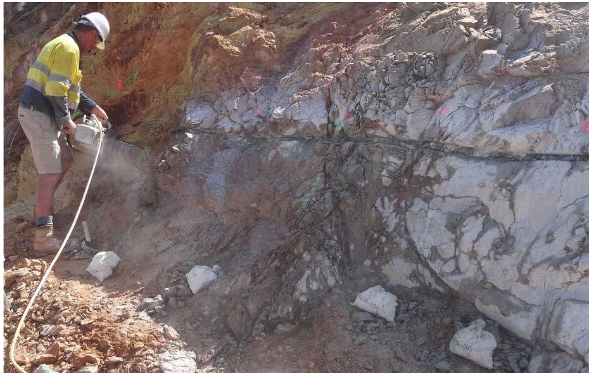
Figure 14 : Diamond saw rock channel sampling AQH – November 2014
