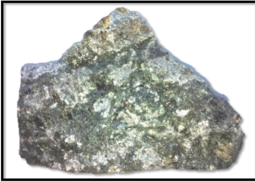
Brecciated Dacitic Porphyry with disseminated chalcopyrite and chalcocite from the base of the Carmelita workings (~50m below surface) on the eastern edge of Target 1.
