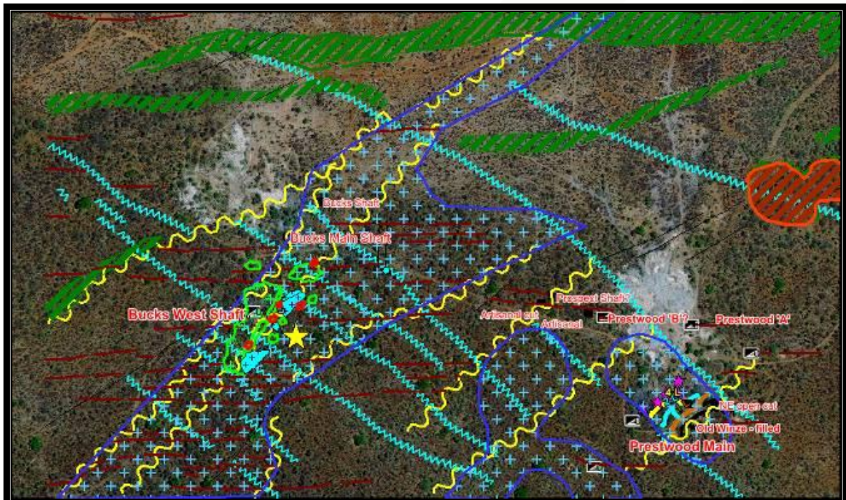
Figure 3: Position of the current artisanal activity (yellow star) superimposed on the geological model. The newly active artisanal zone extends for almost 200m along a shear
