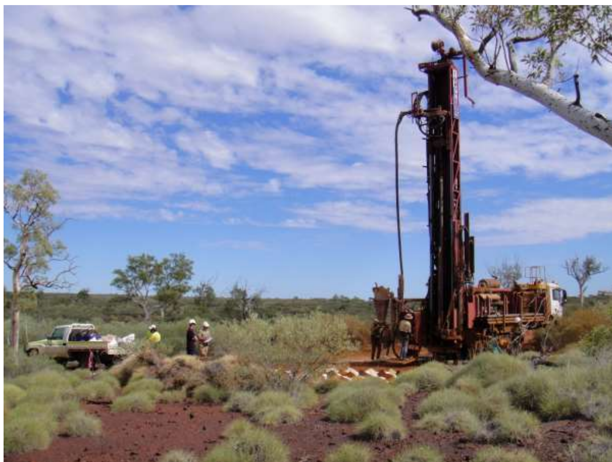
Fig 1 Topdrill Pty Ltd RC rig drilling the Robe Mesa.
