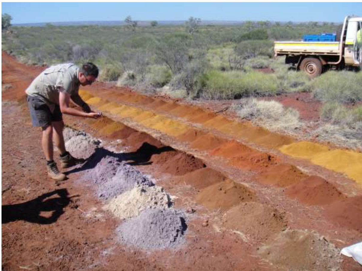
Fig 3. Geological logging of 1m interval samples from the Robe Mesa contrasting the lighter coloured basement (fore-ground) from the overlying intervals with pisolitic iron-stone.
