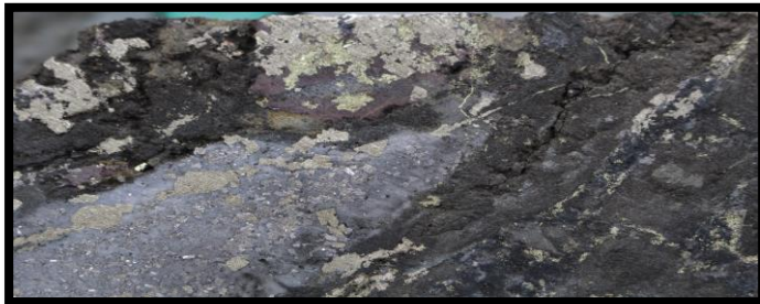
Figure 4: Core photo at 286.8m in CH-DDH013. Pyrite and arsenopyrite occurring in a breccia clast encased in a tourmaline rich matrix containing pyrite and chalcopyrite, as replacements and veins. The metre sample of this section of core returned 1.71% copper, 0.66g/t gold and 72.9g/t silver.
