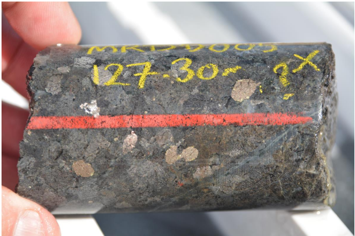
FIGURE 2: Core from MRDD005 showing globular sulphides at depth 127.3m.
