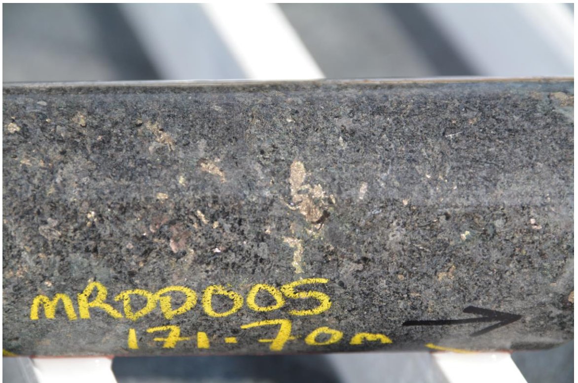
FIGURE 4: Core from MRDD005 showing blebby sulphides at depth 171.7m.
