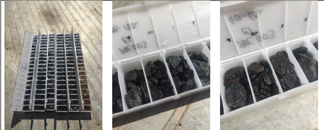
Figure 3: RC chip trays from PRC003 showing mafic rock samples
