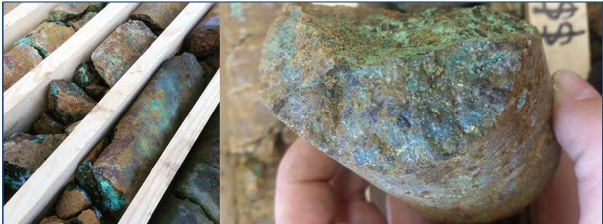
Figure 2: Photo on left-hand side showing pervasive secondary copper mineralization and strong iron oxide alteration. Photo on right-hand side showing primary chalcopyrite mineralization in addition to the secondary chrysocolla mineralisation. Both photos show core from PADH15005 between 48.5-50m downhole.
