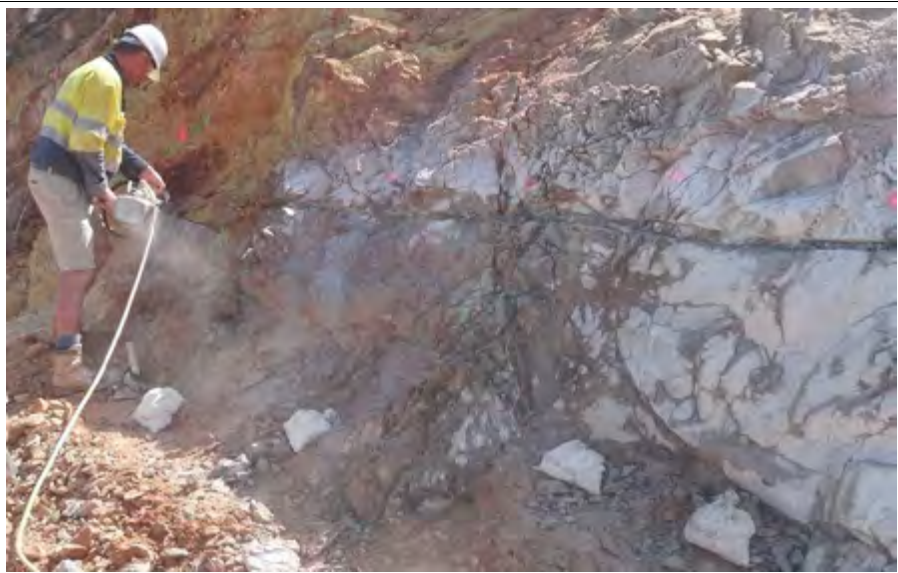
Figure 14 : Diamond saw rock channel sampling AQH – November 2014
