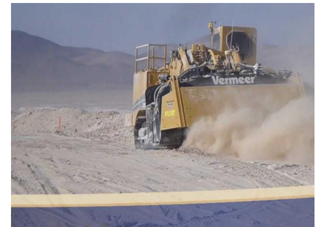
Salt extraction using surface miners
