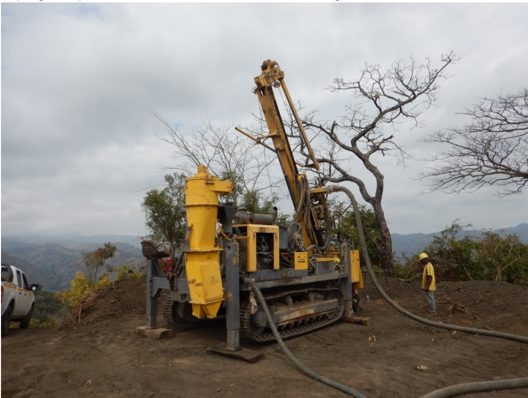
Photo 2. RC drill rig setting up over hole RC44 at Cascade prospect
