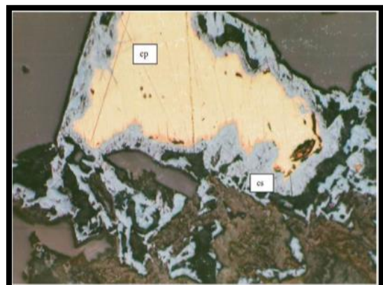
Figure 1b) Thin-section photomicrograph of copper sulphides from the adjacent rock sample.
