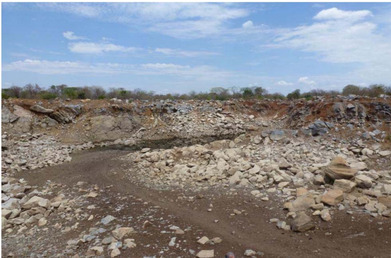
Figure 3. This existing quarry has been mined to 10 metres depth for road base – sampling shows it contains cement grade limestone and that the mineralisation is open in all directions and at depth.
