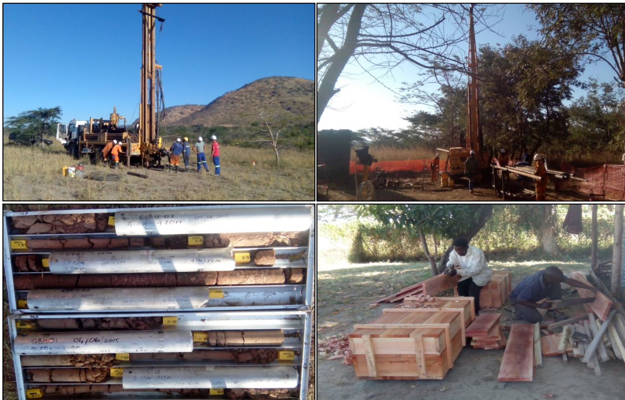
Figure 2: Showing hydrological drilling near the base of Panda Hill (top left), drilling for geotechnical samples in the TSF region (top right), geotechnical core samples (bottom left) and carpenters preparing boxes to transport the samples to South Africa (bottom right).
