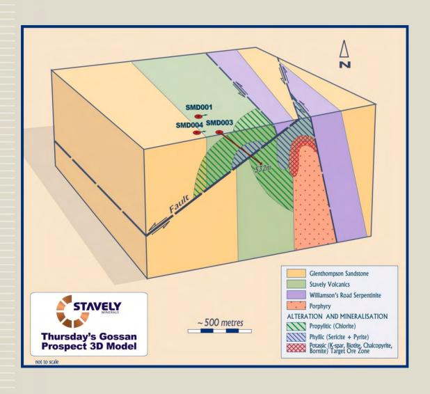
The three deep diamond drill holes identified a low-angle structural offset to the porphyry system
