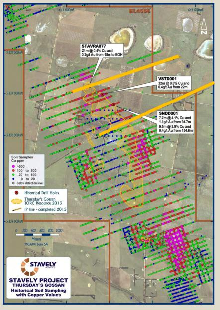
New IP survey lines to extend coverage to east and north where structural model say the target porphyry 'core' has been transposed
