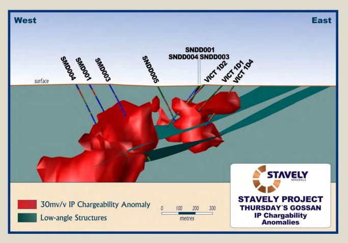
Drilling intercepted well-developed phyllic alteration (sericitepyrite) which corresponded well with the IP chargeability anomaly
