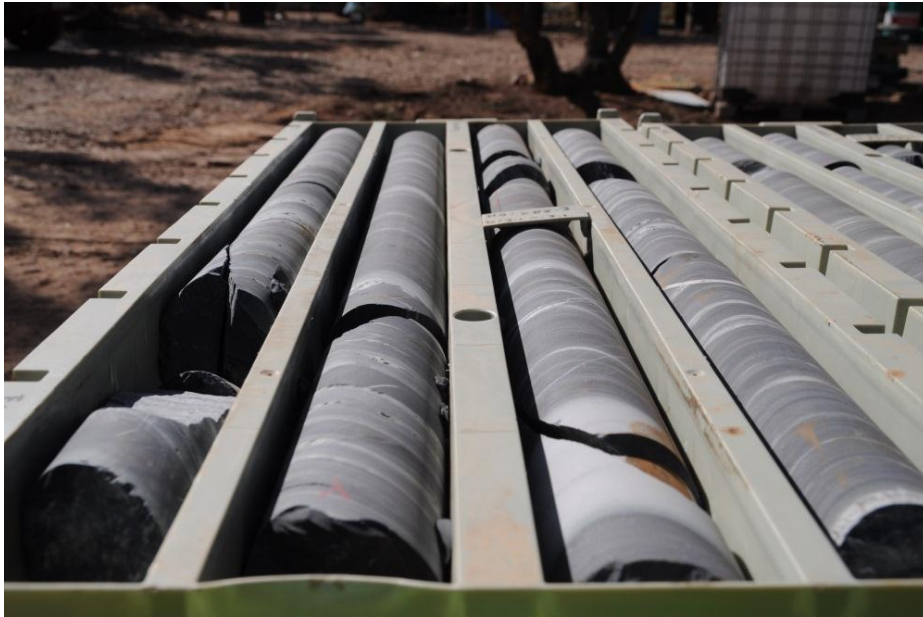
Figure 11 - Magnetite iron ore core samples.
