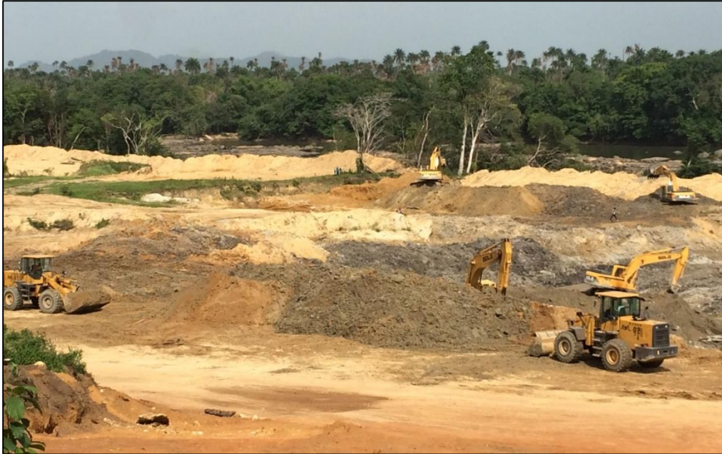
Photograph 3. Pre-stripping and mining activities in the Golu trial-mining pit, Baoma District. Note: a previous bulk-sample trench, excavated to test for mineralisation, lies at the top of the photo (green, grassy area trending left to right.) The tree-line marks the bank of the Sewa River.
