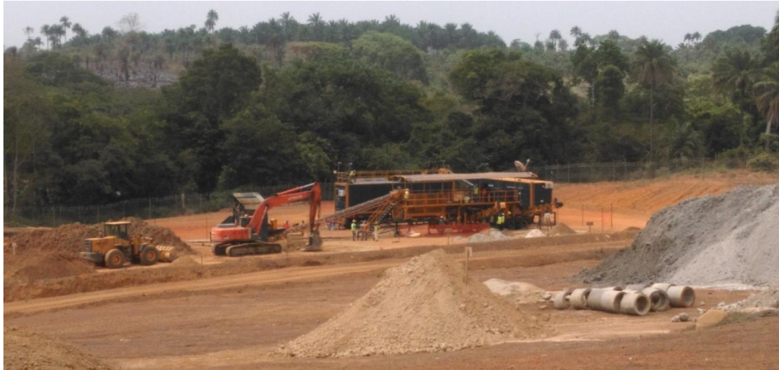
Photograph 2: Allotrope's Diamond Project, Sierra Leone – Exploration bulk sample stockpiles in foreground and DMS plant in background
