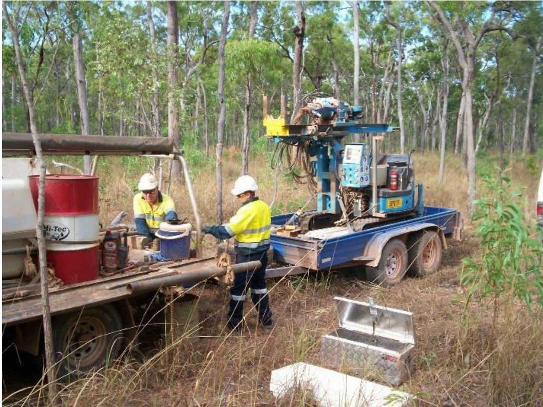
Figure 4: Photo of the sonic drill rig set up
