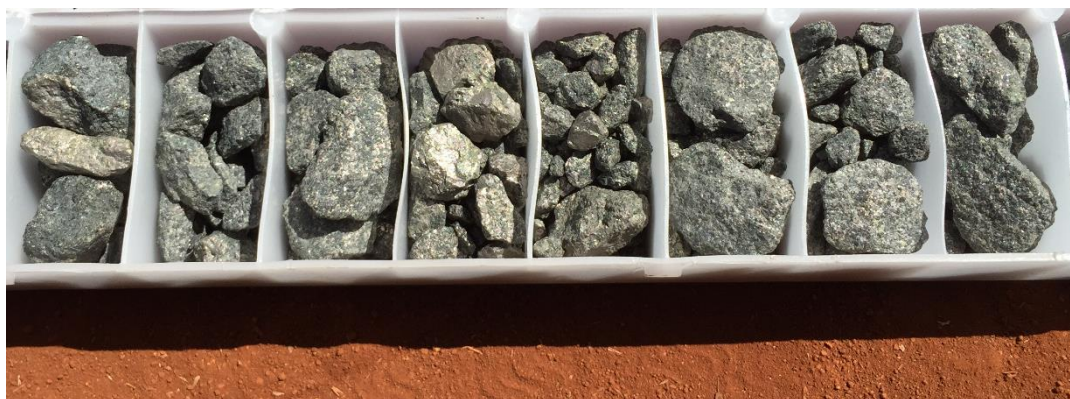
Figure 5. RC chips from the massive and matrix sulphide zone, from 50-58m in hole DMRC0003
