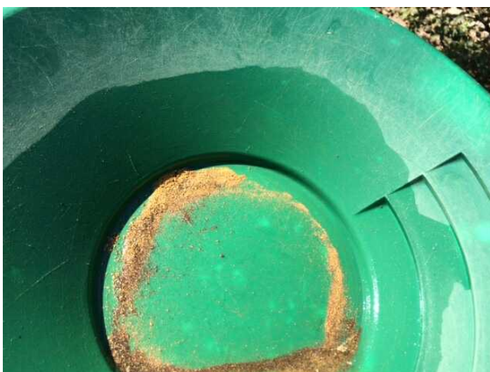
Figure 1 Gold extracted by panning a crushed 100kg sample extracted from the Southern Gold Zone.
