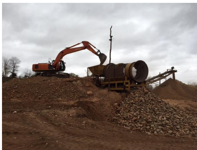
Figure 3: Hitachi Excavator and Rotary Screen in operation
