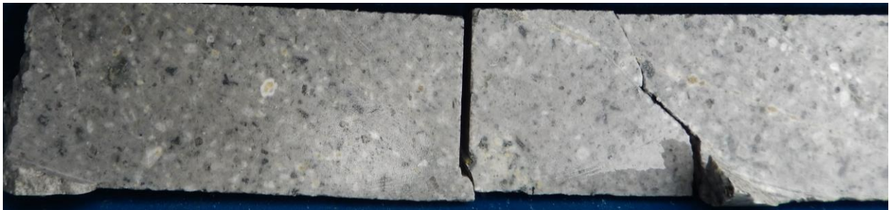
Figure 4: ABOVE Core photo at 534m (CH-DDH027). A silicified quartz monzonite porphyry with minor sulphide veins. The pale coloured quartz growths (eyes) are characteristic of this type of porphyry.
