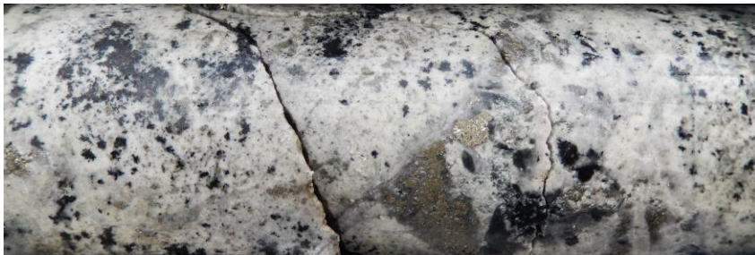
Figure 3: LEFT Core photo at 587m (CH-DDH027). The monzodiorite is highly altered (phyllic) with tourmaline rosettes and sulphide replacements. The sulphides occur as patches, veins and as disseminations.
