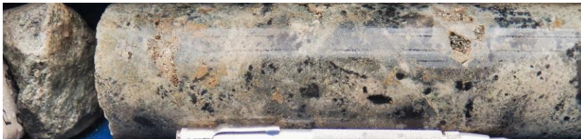
Core photo @ 571m Completely altered sulphide-bearing monzodiorite porphyry CH-DDH027
