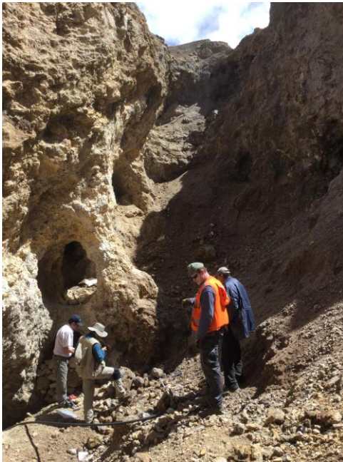
Figure 6: ABOVE The Wari Mine provides direct access to the Zn-Pb vein system, which is up to 5m across.
