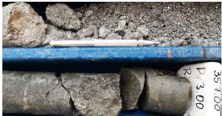
Figure 2: RIGHT Core photo at 357m (CH-DDH027): Massive to semi-massive sulphide zone.
