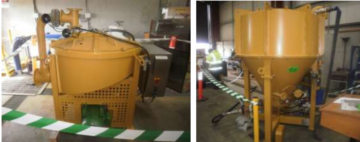
Figure 2 – Pressure Jig – high mass pull gravity gold recovery (left) and In-line Spinner – centrifugal gravity gold recovery at Gekko Systems in Australia
