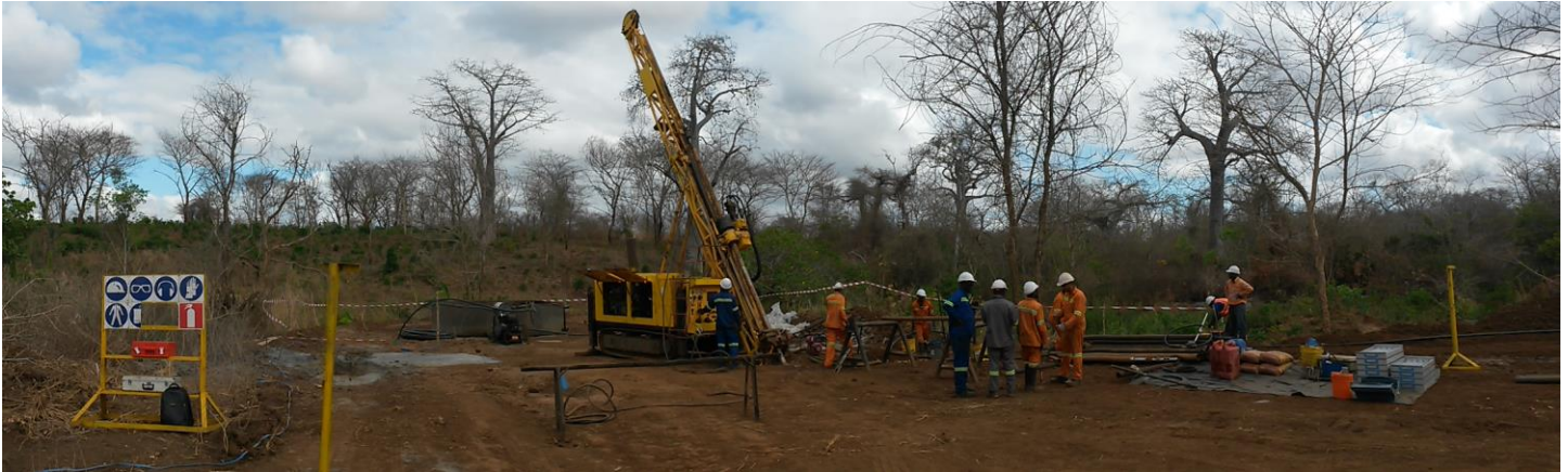
Photo 1: Diamond drilling at Lindi Jumbo graphite project DD hole number LJDD001
